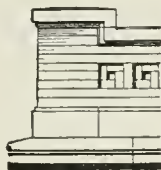
PARAPET: MODERN PATTERNS IN BRICKWORK, WHICH MUST BE CAREFULLY LAID IN STRONG CEMENT MORTAR.
